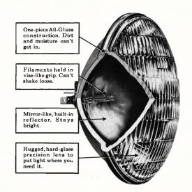
WHEN YOU BLOW ON YOUR GLASSES, moisture condenses on the lens. When moist air gets inside some types of sealed-beam headlamps, the same thing happens. It condenses on lens and reflector. And as the water deteriorates the reflector, the lamp grows dimmer.
