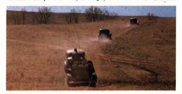
Jalopies roar over plains toward hunting area. Most have reinforced springs and doors welded shut to help them withstand terrific pounding of the chase
